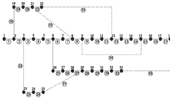
Fig. 1. IEEE33 node structure diagram
